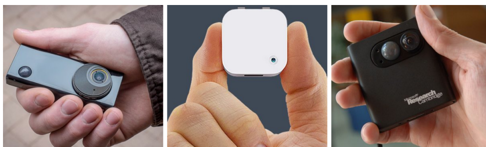
Figure 1: Three lifelogging devices: the Autographer, Narrative Clip and SenseCam.
